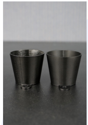
Made of ABS by FFF
